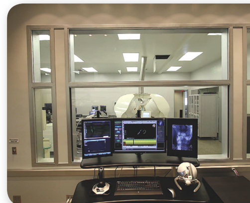
CGCI is operated from the control room or the operating room. Remote Web-based interfaces are not yet available or approved by regulatory authorities, but are likely to become a reality, enabling robotic surgery to be performed from anywhere in the world. Source: Siemens
