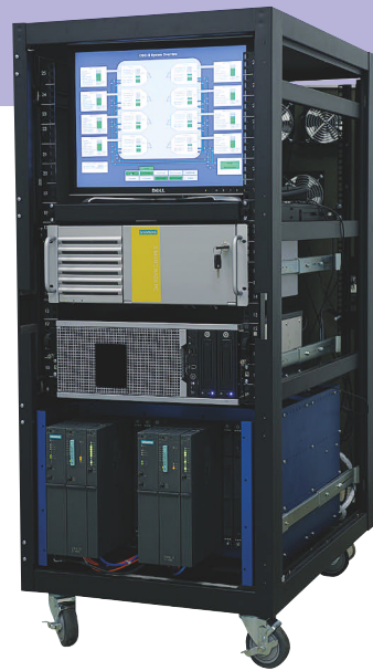
Magnetecs chose a Simatic S7-400H PLC from Siemens to provide automated and redundant safety monitoring, and smooth startup and shutdown of the CGCI system. Source: Siemens
